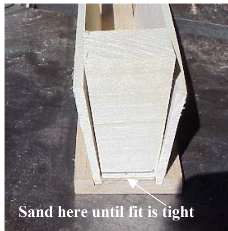
Test fitting the end blocks
