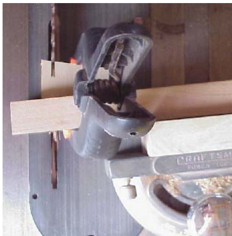
Cutting the blocks to length
