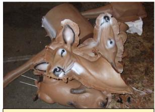
Recently made targets waiting to be trimmed. The painting is done in the mold, and then captured in-place when the foam fills the mold.
