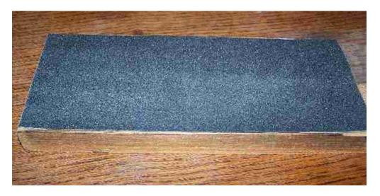
Step 5 Cut up a bit of inner tube to make non slip feet for your board. Glue into place. Using a permanent marker, write the grit size on your board
