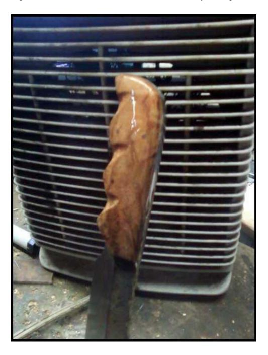
I did a hand sanded finish on the blade so I clamped it back into the vise using leather to cushion the handle and started with 400 grit and worked my way to 800 grit. The trick to a pretty hand sand is to finish it sanding in one direction only; never back and forth. Move your sandpaper toward the handle, pinch the edge and pull toward yourself like you're trying to wipe oil off the edge with your fingers. It takes time but it's pretty when you're done.
