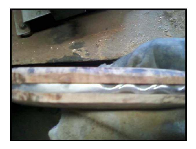
When you're sanding the handles move around a lot, switch from one side or area to the other a lot to keep any one area from overheating. If you overheat a pin it will burn the hole and have a dark ring around it all the way through! You can see the dark areas above where the Cherry burned.
