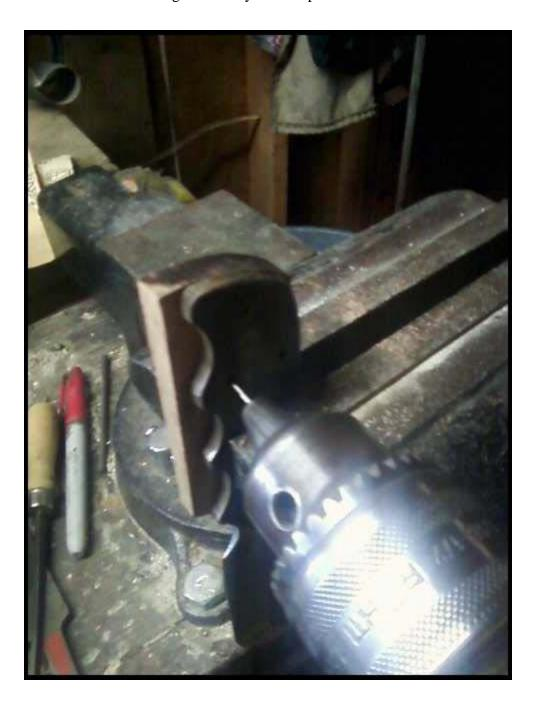
Now, clamp the two scales together to where the front edges match perfectly and CAREFULLY use the first scale as a template to drill the holes in the second. This way they're sure to match.
