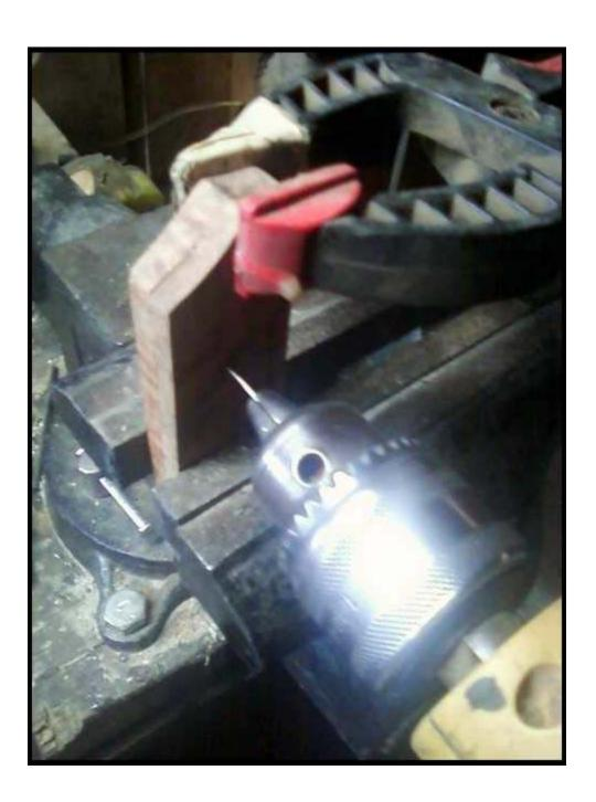
I FORGOT!! You need to use a drill bit that's just a tad smaller than the pins when you drill the scales so they're fit nice and snug.
