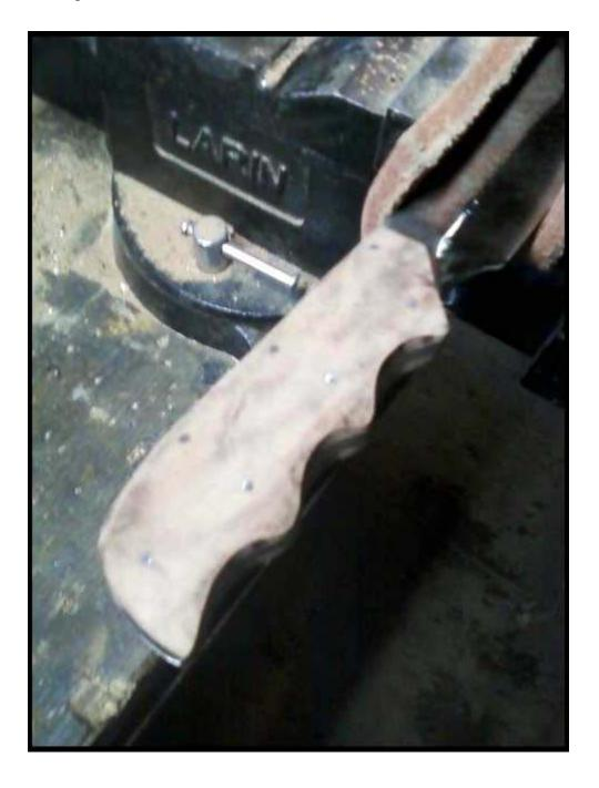
To make the finger comfort grooves on this one I first used a small round edged file, then a magic marker wrapped in smaller and smaller grits of sandpaper.
