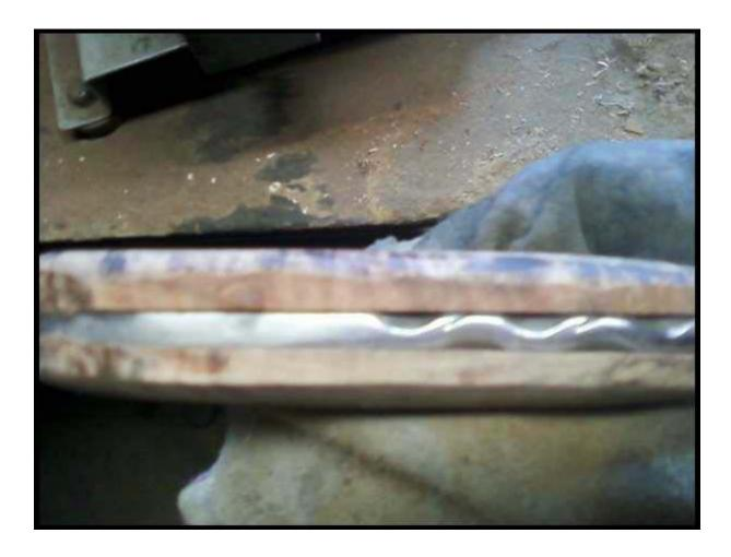
You can rough shape the handle with a rasp but you have to avoid the pins or it will ruin the rasp and handle. A file works too, but heavy sandpaper and a sanding block work best if you don't have a power sander of some sort.
