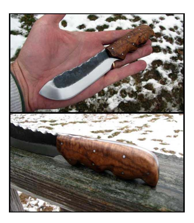
Left out a step on the file work. Once you get the grooves ground go back with the edge of a bastard file or a triangle file and file marks in toward the opposite side of the knife (see drawing). Once this is done lightly file the edges of the bigger grooves you made earlier so that they have a rounded look and thus form the "vine look". Is that as clear as mud?
