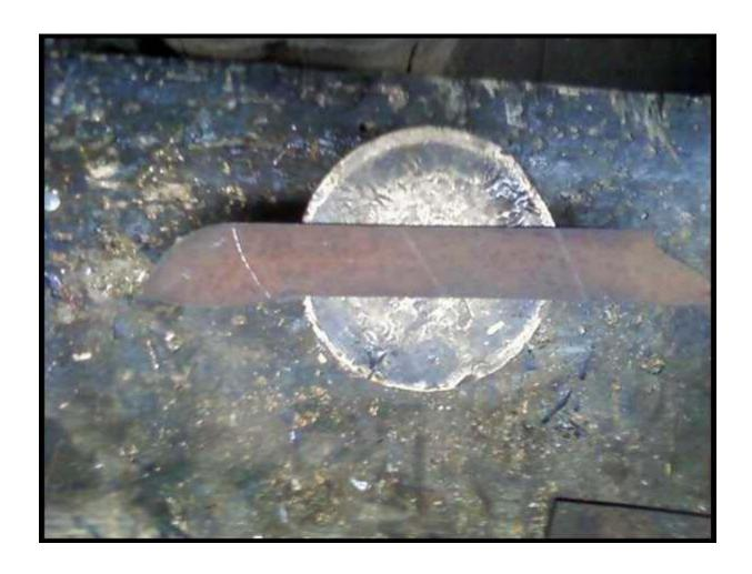
I ground the end of the blade to shape with a grinder and stone wheel; kind of a mini nessmuck shape. Then I took a regular magic marker and marked out where I wanted the finger grips to be. Then I ground the shape into the steel with the same wheel.
