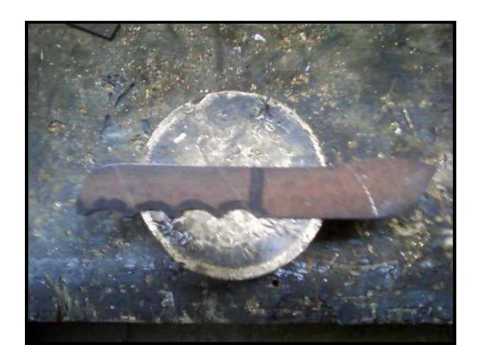
Then I taped off where I wanted the edge to be. This helps in two ways; it helps you keep up with where you're ground and it keeps you from scratching the other part of the blade if you don't want to. I eyeballed the width of the edge, I just know where I want it to stop, yours could be different.
